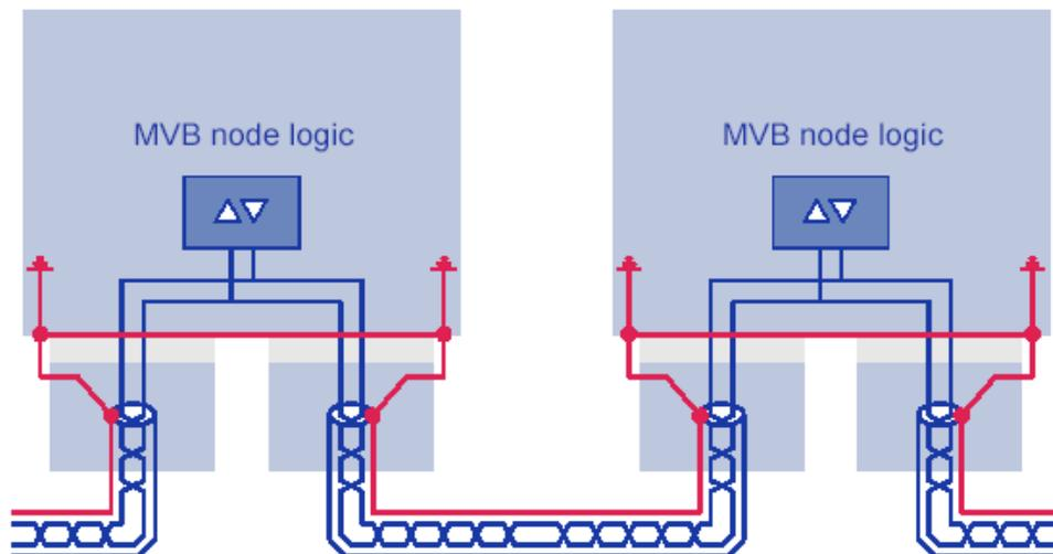
As a result, all housings are connected together. Within the vehicle concept it must be ensured, that there are no ground potential differences that may harm the cable shield or the connectors.
