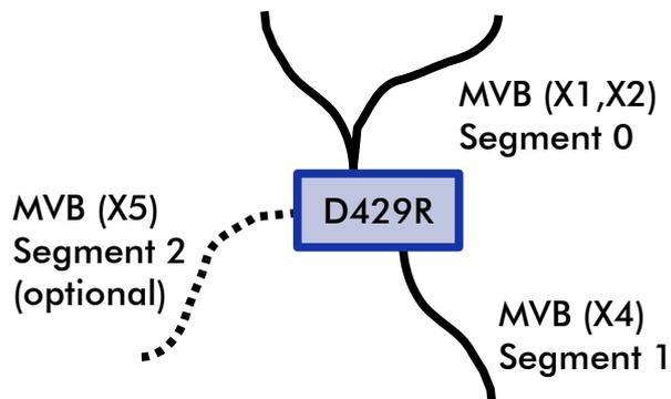
As an alternate option the D429R can be used to connect three MVB segments together (star coupler). The segments 1 and 2 are connected at the end of the line or via a T-stub to X4 and X5, respectively.
