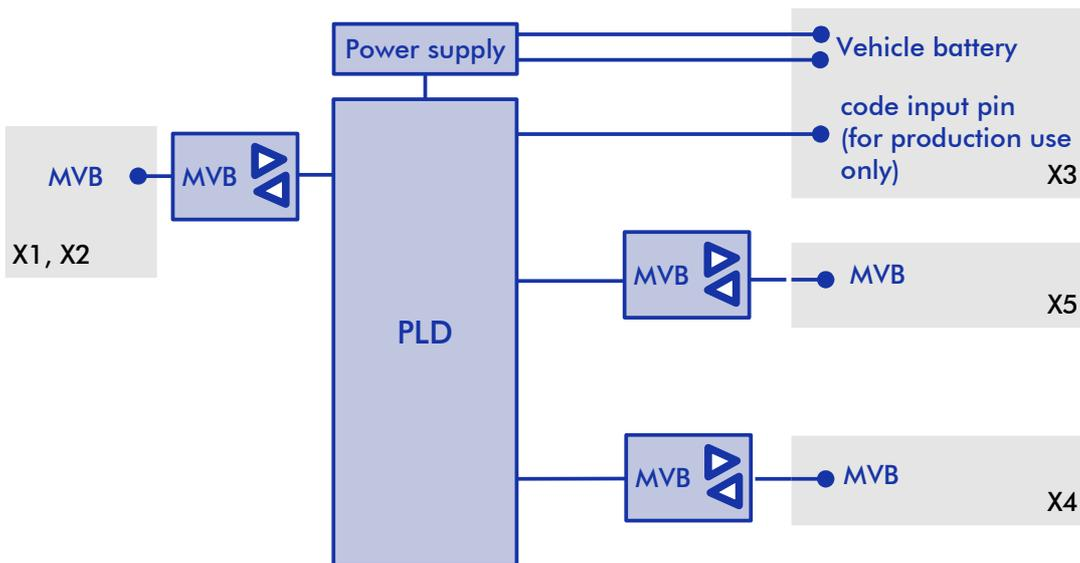
The PLD programmable logic includes several functions like the Duagon **MVB controller** and several other peripheral digital functions. Depending on the application, it is compiled matching to the set of used hardware options. **Power** is drawn from the vehicle battery supply. This includes the supply for the various communication transceivers as well as the internal logic.
