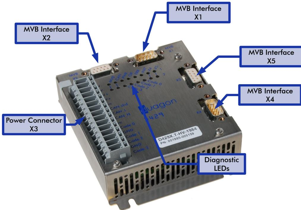
The figure below shows the D429R. Basic Function Blocks
