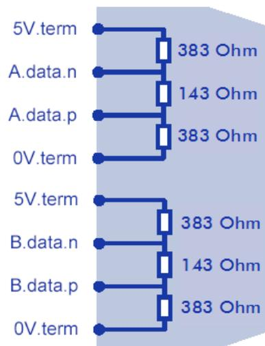
In case the D429R is the last of several MVB nodes, one of the D429R- MVB connectors remains open. The terminator is mounted on this connector and delivers the correct line termination.
