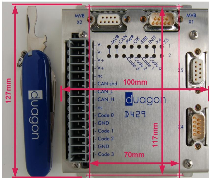
The picture below shows the "height" of the D429R case without connectors (all dimensions in mm).
